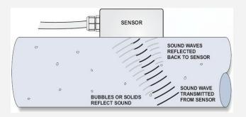
The proprietary onboard processor performs a spectral frequency analysis of the waves to calculate a flow profile. From the profile of these sound waves, a mix of on-board and cloud-based algorithms compute a fluid velocity in the pipe.
