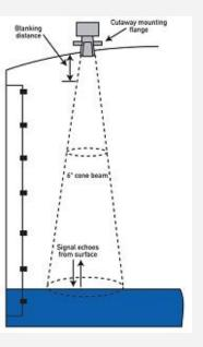
The proprietary onboard processor examines the millions of waves that return to the module, and examines the amount of time each wave takes to return back.
